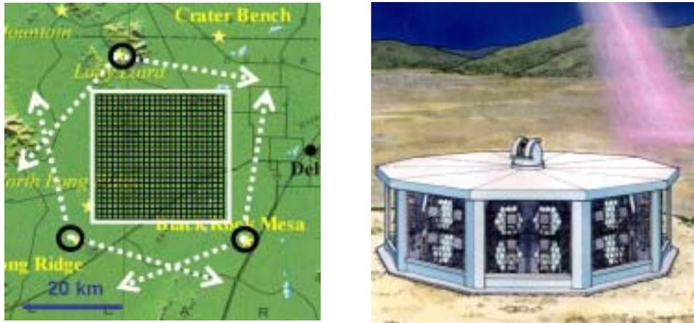
**Fig. 1.** The Hybrid TA (left panel) is composed of 576 plastic scintillation counters covering the ground area of  $760 \text{ km}^2$  and 3 fluorescence telescope stations (right panel) surrounding the ground array and looking inward.
