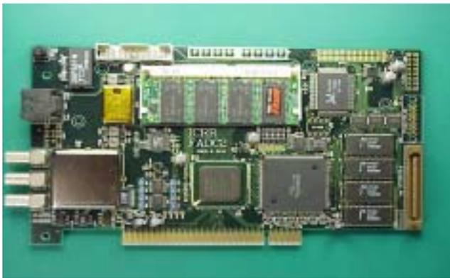
Fig.2 Prototype Flash ADC Board
