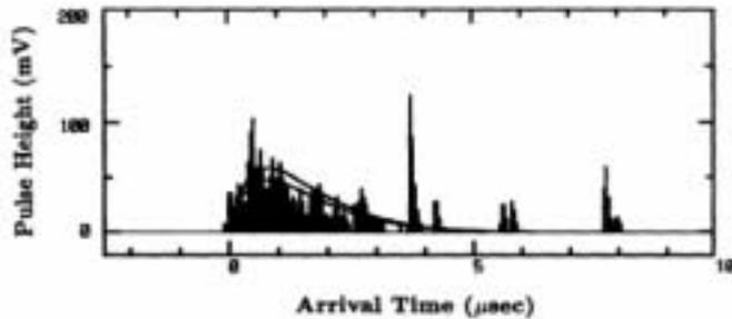
Fig.3 Time profile of 30 m<sup>2</sup> scintillation counter signal observed 2 km away from the shower core of a large air shower event ( $E=2 \times 10^{20}$  eV) observed by AGASA.
